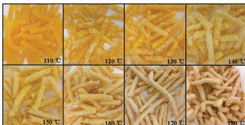
Figure 3. Appearance of the extruded products from wheat grits by screw 1/1 at 110–180 °C.
